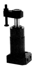
work supports and these new hydraulic clamping elements offers high clamping or retention forces at low pressure. All operate at 70 bar pressure and are designed to offer short clamping times. The clamping elements are also compact so ideal for use when space is at a premium and all are available with position monitoring if required. The entire range is fitted with metallic wiper seals to reduce maintenance and increase durability.
