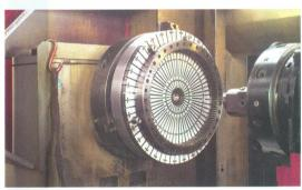
reliably clamp even rough workpieces, as it can overcome any gaps between the workpiece and the chuck. The control unit allows the magnetic force to be varied to suit the application and operation can be manual, automatic or combined, and chuck sizes can be matched to suit the workpiece.
