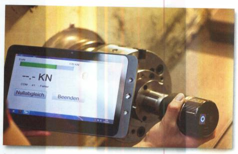
that the actual clamping force is known. Using the TESTit gauge the clamping force can then be calibrated to exactly match the process requirements."
