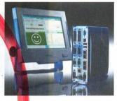
The Type 5847 maXYmos NC from Kistler will monitor, evaluate and document the XY characteristics of joining and press-fit processes using force and displacement data from a servo press module.
