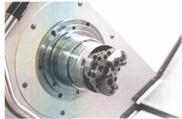
The basic unit is a Spanntop collet chuck or Toplus collet chuck. Add to this the jaw module, clamping heads and mandrels, and users achieve reliability, accuracy and safety that traditional jaw chucks lack,
