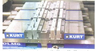
into the side of the master jaws, and are secured via clamping elements that provide downward pressure to keep the jaws in place. Jaw change takes less than
