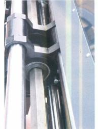
the use of reduction tubes in the lathe spindle and polyurethane bar retaining sleeves that spin on ball bearings mounted on fixed and moving steadies.
