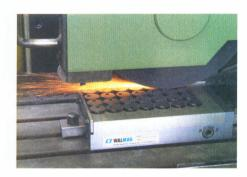
install and can be quickly transferred between different machines if required. A permanent magnetic system does not generate any heat so there is no risk of thermal deformation of the pole plate or the workpiece, helping to maintain machining accuracy.
