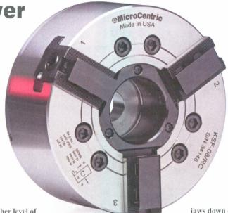
If a higher level of accuracy is required after the top jaws have been changed, the radial-run out of KSF chucks can be adjusted; because the spindle adapter mounts to the spindle nose and the chuck then mounts to the adapter plate, the radial-run out of the clamped part can be corrected to between 10 and 20µm using four adjusting screws on the outer diameter of the chuck body. Furthermore, a wedge design that securely pulls the
