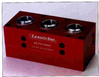
Featuring a compact design with three closers integrated into one body, the Tri-Grip unit has simplified hydraulic plumbing and an accessible-from-the-top collet locking screw that allows the part to be correctly orientated. With a maximum working pressure of 5,000lb/in² and a draw-tube force of 1.1-
