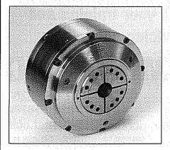
Clamping force is adjustable by tightening or loosening the collet using the spanner holes in the front of the collet. For fragile materials or thin walled parts the clamping force can also be reduced by removing pairs of springs inside the chuck.
