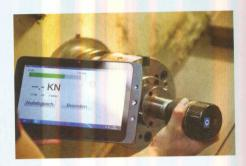
machining process. Using the new TESTit clamping force gauge the efficiency of any fixturing will be maximised. If you cannot measure something, you cannot control it, so specific clamping measurement data should be demanded by industry," concludes Mark
