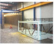
8m wide x 8m high and can accept loads to 40t. Double doors at one end provide a 7m x 7m opening. Walls and roof are constructed from prefabricated mild steel panels covered with full-height rubber curtains. The concrete floor is protected with steel plate to retain a smooth, safe surface. Two personnel doors have been fitted and all doors are interlocked with the blasting system to prevent it being used if one is open.
