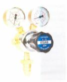
ESAB oxygen regulators incorporate built-in Regulator Burn-Out (RBO) protection, which contains oxygen regulator fires when used properly. Oxygen regulator bodies are machined from solid brass bar stock that provides a thick wall that helps contain a burnout. With the size of internal body cavities kept to a minimum, the amount of gas that can accumulate is limited. The solid design also contributes to the durability of the regulator.
