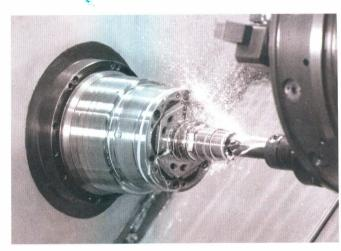
For radial clamping without axial movement of the clamping head the deadlength TOPlus Mini is suitable for component transfer between spindles such as horizontally opposed twin spindle lathes, also known as kissing-spindle lathes, and for vertical turning pick-up spindles. Again, the chuck can be used for through-bore work with bar fed raw material.
