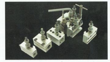
A variety of toolholders are available to take square and vee, parting, boring and Morse taper bits, which, once mounted in place on the central block, can be quickly adjusted in height until the best cutting effect is found and the setting is locked.
