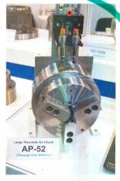
guarantees safe operation up to maximum speeds that extend from 4200 rpm for the AP-52 to 3000 rpm for the AP-115.
