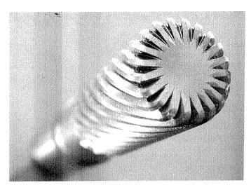
tool flutes to break up harmonics and reduce chatter. "Titanium is very prone to chatter, which affects part quality, and can cause unpredictable tool failure," said Grubbs. "By using extremely high feed rates and light radial cuts, we can remove a lot of material with very little risk of scrapping parts."
