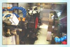
release their capacity for more suitable parts. It really is the ability to overlap the machining of features on the BNJ making full use of the 'butterfly' second turret that is making us so competitive in that new area."
