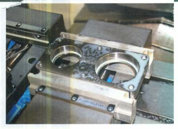
carved jaws will repeat  $\pm 7.5 \mu m$  when replaced in the original master jaw. Operators can dowel pin the aluminium jaws ready to be reused or purchase SMARTstopped (pre-pinned) 4" and 6" jaws in all five aluminium profiles, 1018 or ductile cast iron jaws.
